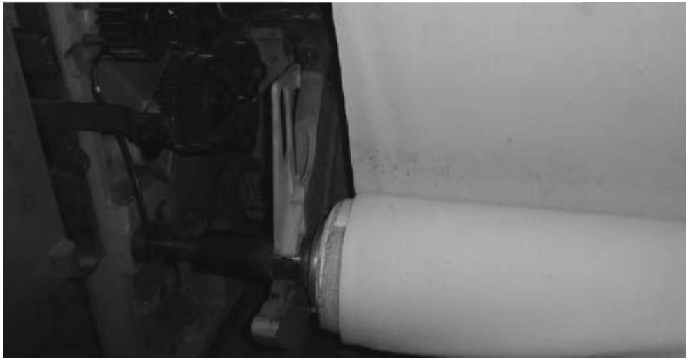
Figure 9: Take-up mechanism on loom.
