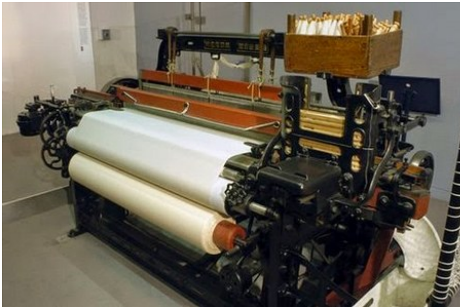
Power loom used in weaving factory
